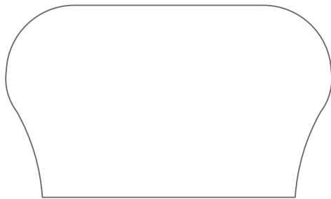
28 HANDRAIL 1 7/16" x 2 3/8" - no/plow
